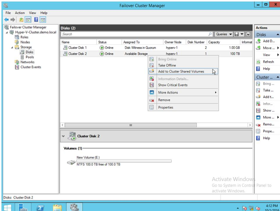
On the bottom pane, the 100 TB disk volume will change from NTFS to CSVFS (Clustered Shared Volume File System), this allows the volume to be used by many Hyper-V nodes concurrently. Notice too that it is now accessible as “C:\ClusterStorage\Volume1”.
