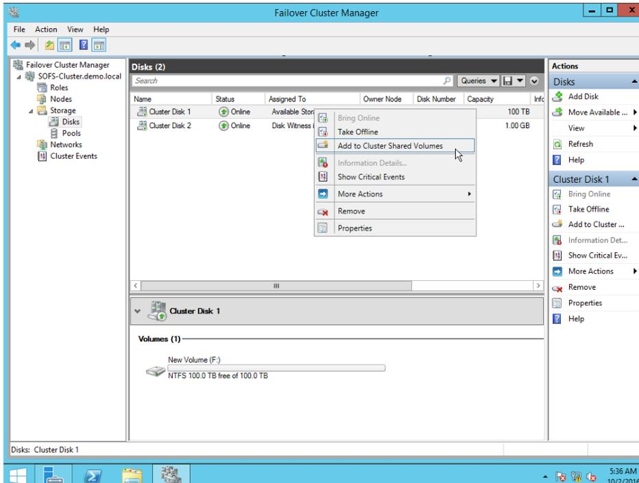
On the bottom pane, the 100 TB disk volume will change from NTFS to CSVFS (Clustered Shared Volume File System), this allows the volume to be used by many SOFS nodes concurrently. Notice too that it is now accessible as “C:\ClusterStorage\Volume1”
